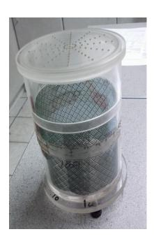
**Photo 2A**. The custom made Perspex test cylinders used to determine the TP, CC, AFP and DBD of the raw materials and growing media mixes. The capacity of the test cylinders was 1L± 0.03mls and based on the design of Byrne and Carty, (1989)
